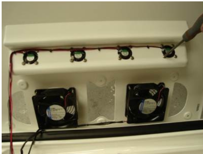
Figure 17a: Evaporator fans
