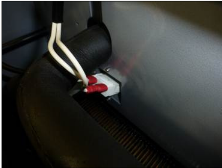
Figure 15: Spade connectors connected to the drawer switch
