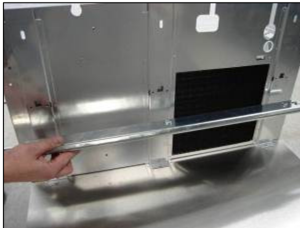
Figure 24c: Fixings in vertical wall supports and lancing's in runner outer beam
