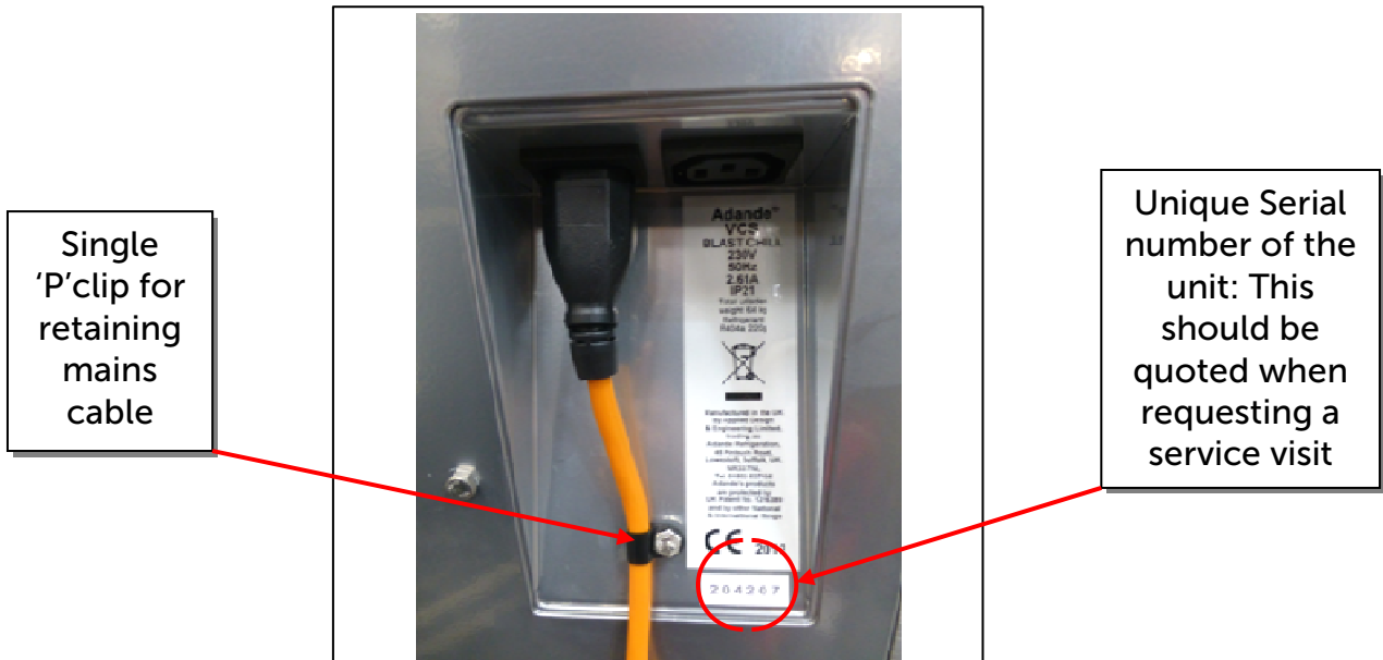
Figure 3a: Mains connection point
