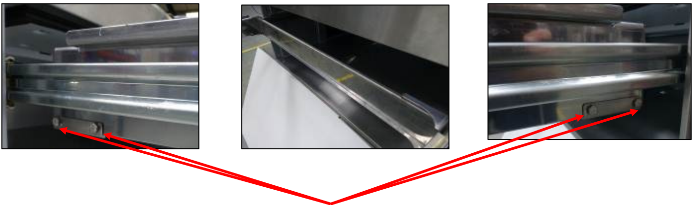
Figure 23a: Brace container support rear and four off M5x8
